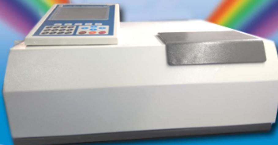
2203 is a  $\mu$  controller based double beam instrument, with varieties of measuring / operating modes, data processing / analysis abilities, system optimisation / self diagnostic / calibration utilities etc.
